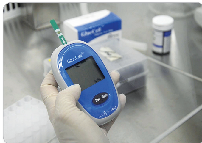
Fig. 2: Portable meter and disposable test strips enable the operation in a biosafety cabinet.
